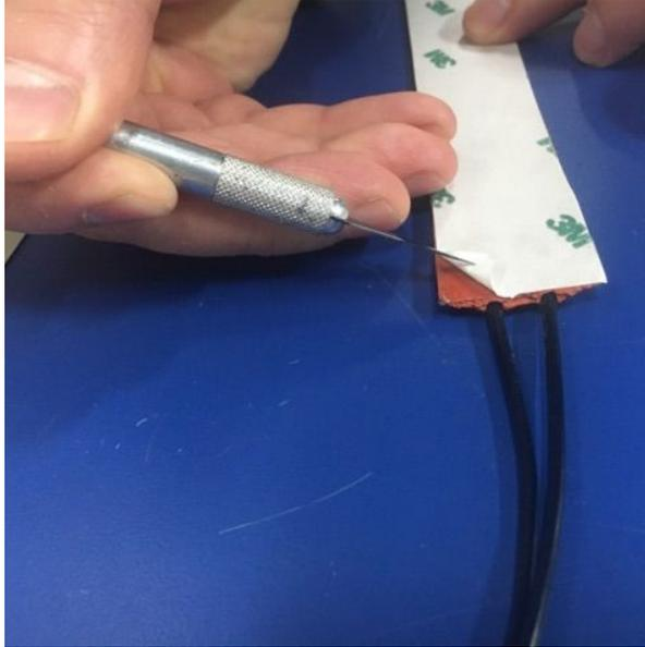
3. Grab the corner of backing paper and continue peeling it back, along the surface, to expose a few inches of PSA. Do not touch PSA, especially at the edges:
